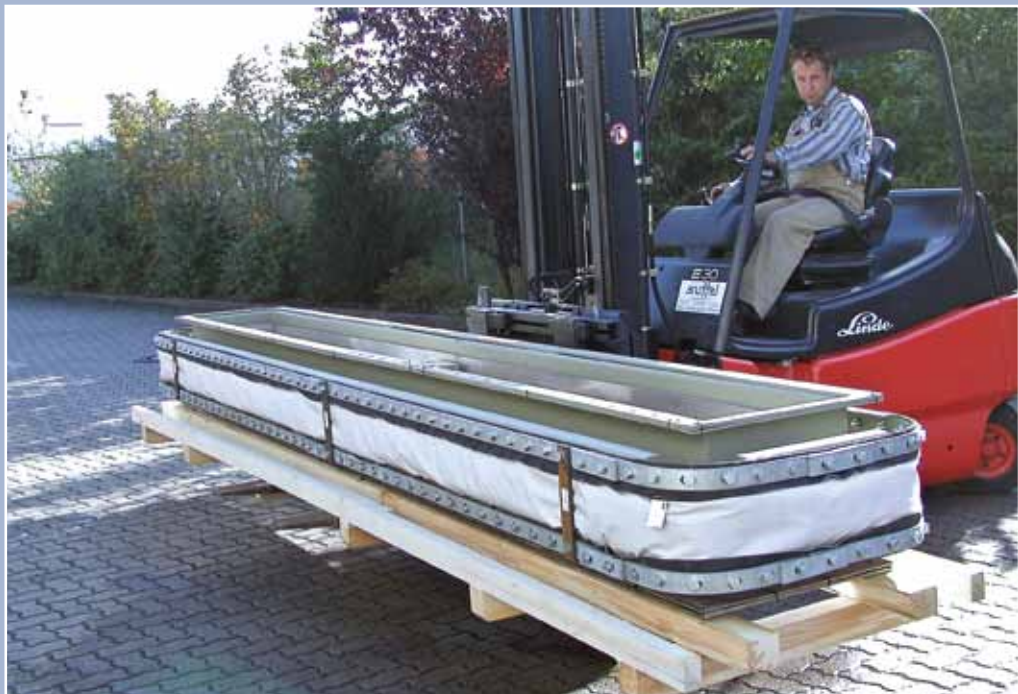
Multilayer expansion joint, type GB300 as a pre-fabricated installation unit for ash discharge in a power plant NG 5500 x 600, 750 °C
