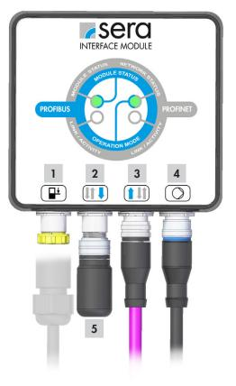
The field bus box modules are connected via the supplied connection cable. The INTERFACE MODULE has a socket and a plug, whereby no Y-connector is necessary. The supply voltage (+5 V DC) for the terminating resistor is only applied on the socket. The terminating resistor is only available as plug connector.
